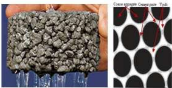
Gambar 5 Gambaran dasar No-fines aggregate concrete
